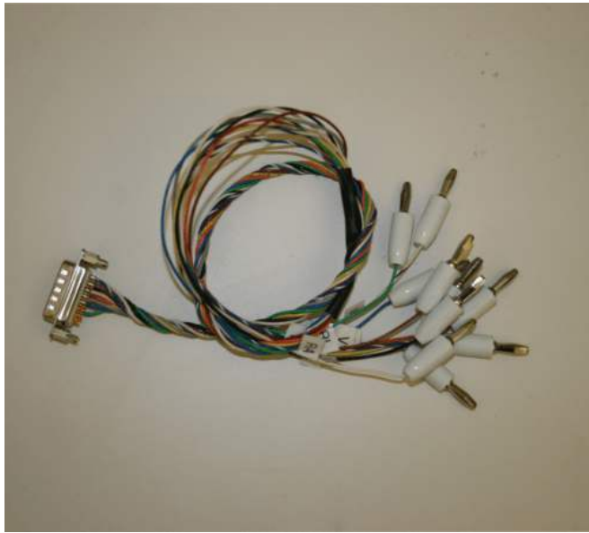
Figure 46. 15-Pin, Twisted Wire Cable to Banana Jacks
