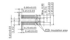
Recommended metal mask pattern Metal mask thickness: When 150 µm (Terminal opening ratio: 49%) (Metal-part opening ratio: 100%)
