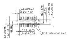
Recommended metal mask pattern Metal mask thickness: When 150 µm (Terminal opening ratio: 49%) (Metal-part opening ratio: 100%)
