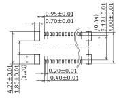
Recommended metal mask pattern Metal mask thickness: When 120 µm (Terminal opening ratio: 60%) (Metal-part opening ratio: 100%)
