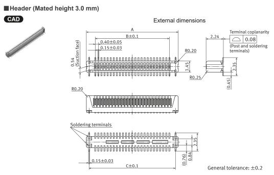
Note: The soldering terminal dimentions of headers with mated heights of 1.5 mm/2.5mm and 3.0mm are different.
