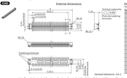
Note: Because the soldering terminal Y and Z are the unified structure, they are connected electrically.
