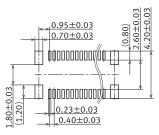
Recommended metal mask pattern Metal mask thickness: When 150 μm (Terminal opening ratio: 48%) (Metal-part opening ratio: 100%)
