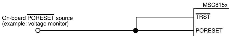
Figure 35. Reset Connection in Functional Application
