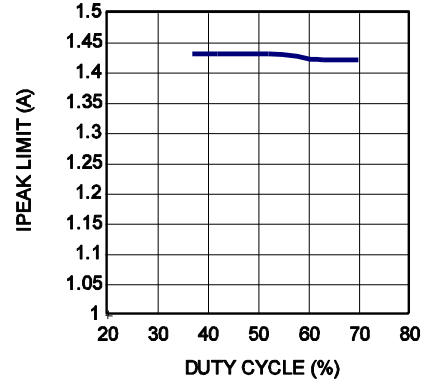
SW peak current limit vs. Duty Cycle
