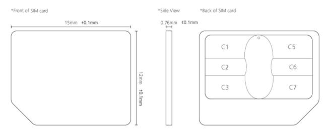
**Note**: The SIM cards Carrier card has tri-cut breakout inserts to allow the SIM to fit into 2FF, 3FF, and 4FF SIM card slots. The mechanical drawing above is for a 3FF SIM card configuration.
