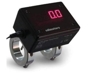
The CDI 5200 clamps onto a pipe, with two flow-sensing probes projecting into the pipe through 3/16-in. drilled holes. It seals directly to the pipe; no cutting or welding is required for installation. Because each flowmeter is made and calibrated for a specific size of pipe, the digital display indicates flow directly, with no setup or adjustment.
