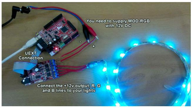
Note that the picture shows RGB that requires 12V DC provided to the PWR\_CON connector. Pin 1 is 12V, pin 2 is GND. In this case UPWR\_E jumper should be open by default.
