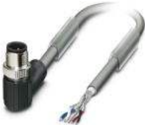
Bus system cable, CANopen®, 5-position, PUR halogen-free, Gray RAL 7001, shielded, Plug angled M12-SPEEDCON, A-coded, on Free cable end, Cable length: 20 m
