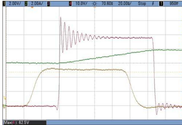
Figure 4: Typical Waveforms for V_{IN} = 48 V to 5 V/7 A (1000kHz) Buck converter CH1: V_{PWM} Input voltage – CH2: ( I_{OUT} ) Switch node current – CH4: ( V_{OUT} ) Switch node voltage
