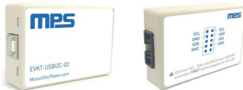
Figure 3: EVKT-USBI2C-02 Communication Interface
