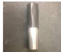
CORRECT ID PLUG GAGE KEEPS TUBING ROUND
