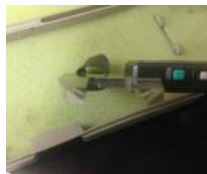
INCORRECT ID TUBING IS STRETCHED
