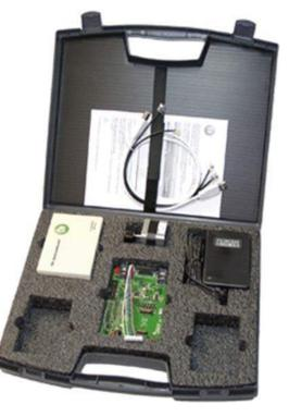
The provided motherboard gives a lot of flexibility during your development process. Easy access to several signals makes debugging very easy and gives you the possibility to connect the evaluation kit with your own application which reduces the development time. Evaluation of the complete NCV7052x family is made very easy by means of the separate daughterboards.
