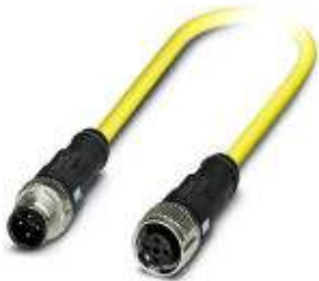
Sensor/Actuator cable, 4-position, TPE, yellow RAL 1021, Plug straight M12 SPEEDCON, A-coded, on Socket straight M12 SPEEDCON, A-coded, Cable length: 3 m
