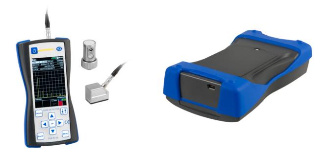
PCE-FD 20 is a portable ultrasonic flaw detector with a large LCD screen that displays A-scan maps of ultrasonic signals as well as B-scan cross sections. Ideal for use in mechanical engineering, aerospace and metallurgical applications, this high-frequency ultrasound-based defectoscope uses a contact transducer (two different probes included; 45° and 90°) to measure material thickness and identify flaws and defects such as discontinuity in welds.
