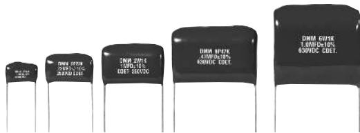
**Type DMM** radial-leaded, metallized polyester capacitors have non-inductive windings and multi-layered epoxy resin enhancing performance characteristics and humidity resistance. Self healing characteristics prevent permanent shorting due to high-voltage transients. When long life and performance stability are critical **Type DMM** is the ideal solution.
