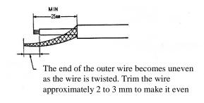
(3) Do not excessively twist the conductors.
