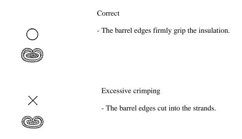
Checking for correct crimping:
