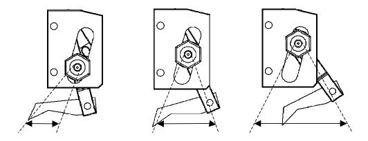
**8-3** When adjusting the pitch always try to feed the terminal on the Insulation bucket as shown in the item 2 below, if this cannot be achieved then using the Conductor bucket is acceptable.
