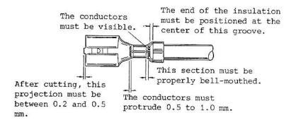
4.2 The crimped cross-section must be correctly finished as shown on the right:
