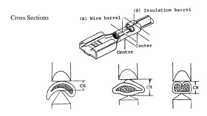
H:\0 - Quality Documents\2 Department\Tech Serv\Application tooling\Applicators and Die sets\TS142-01 CMK-R Manual.doc \* Set the crimp height of the wire barrel to the specified dimension.
