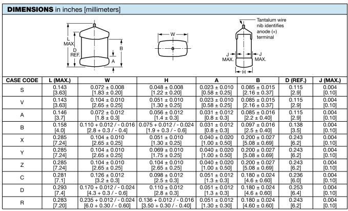
The anode termination (D less B) will be a minimum of 0.010" (0.25 mm)
