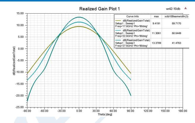
WR-42 Standard Gain Horn with 10 dBi gain, SMA Female connector from Pasternack Enterprises has same day shipment for domestic and International orders. Our RF, microwave and millimeter wave products maintain a 99.4% availability and are part of the broadest selection in the industry.
