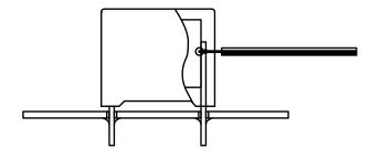
Temperature monitored inside the capacitor.
