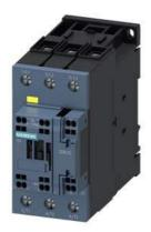
power contactor, AC-3e/AC-3, 80 A, 37 kW / 400 V, 3-pole, 83-150 V AC/DC, 50/60 Hz, with integrated varistor, auxiliary contacts: 1 NC, main circuit: screw terminal, control and auxiliary circuit: spring-loaded terminal, size: S2, F-PLC-IN
