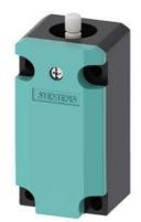
position switch basic switch plastic 40 mm according to EN 50041 increased corrosion protection device connection 1 x M20 x 1.5 1 NO/1 NC quick action contacts functional at -40  $^\circ$ C shock and vibration test according to DIN EN 61373, category 1B
