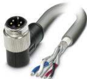
Bus system cable, DeviceNet, 5-position, PVC, Gray RAL 7001, Plug angled 7/8"-16UNF, on Free cable end, Cable length: 15 m
