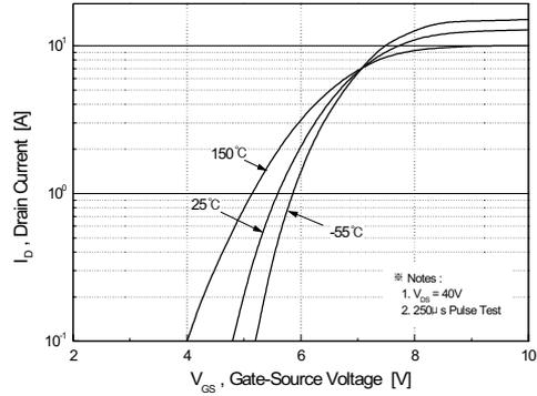
Figure 2. Transfer Characteristics
