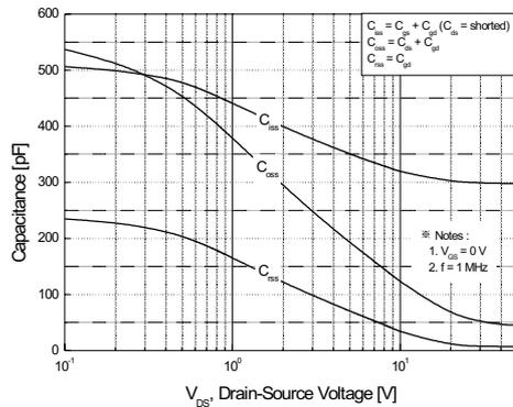
Figure 5. Capacitance Characteristics
