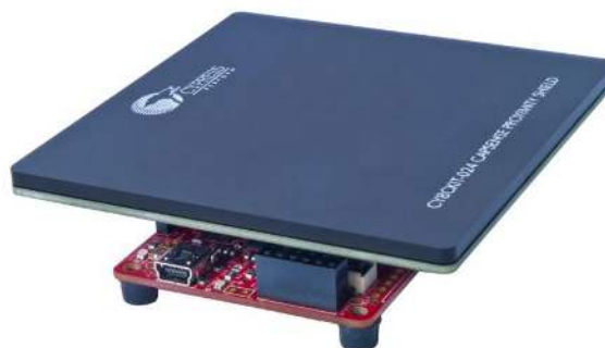
Figure 1-3: CY8CKIT-024 Connected to CY8CKIT-042
