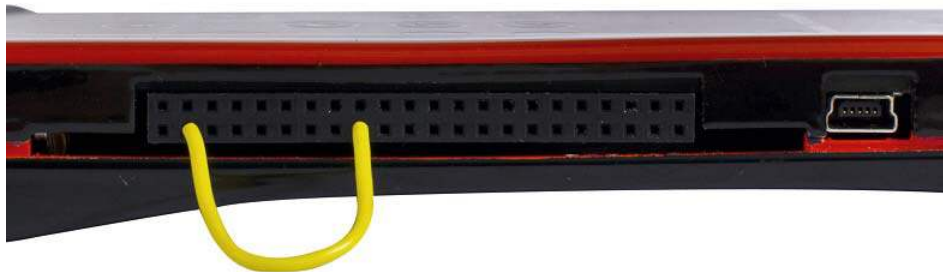
Figure 3-25. Shorting Button #6 (pin #27) to Vdd (pin #41)
