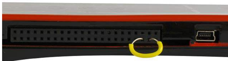
Figure 3-21. Shorting Button #5 (pin #3) to Ground (pin #5)
