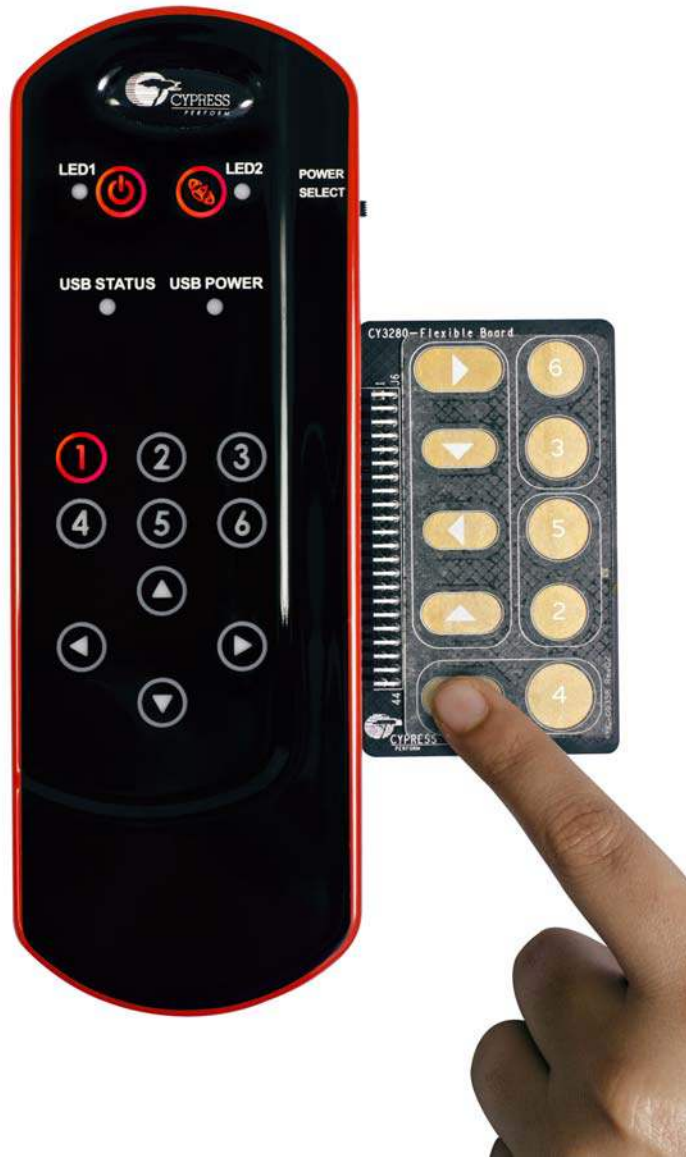
Figure 3-3. Demonstration of SmartSense Auto-Tuning with Flex-PCB
