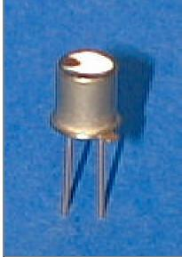
PACKAGE DIMENSIONS INCH [mm] 45 0.50 [12.7] MIN 0.040 0.145 [3.68] 0.189 [4.80] 0.029 [0.74] Ø0.019 [0.48] Ø0.016 [0.41] WIRE BOND DV/////// Ø0.195 [4.95] 0.100 [2.54] Ø0.178 [4.52] ANODE //// CATHODE & CASE PHOTODIODE CHIP Ø0.212 [5.38] Ø0.209 [5.31] LENS CAP 0.025 [0.64] (WELDED) 0.022 [0.56] HEADER 0.027 [0.69] SOLIARE Ø0.012 [Ø0.30] TO-46 HERMETIC CAN PACKAGE ACTIVE AREA ACTIVE AREA =  $0.073 \text{ mm}^2$
