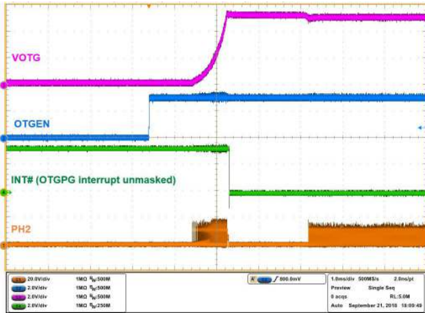
Figure 26. OTG mode enable using OTGEN pin. V_{BAT} = 11V , V_{OTG} = 5V , general purpose comparator disabled, OTGEN Control bit enabled
