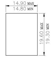
Single Panel—Latch Clearance Panel Thickness 0.062 inch.
