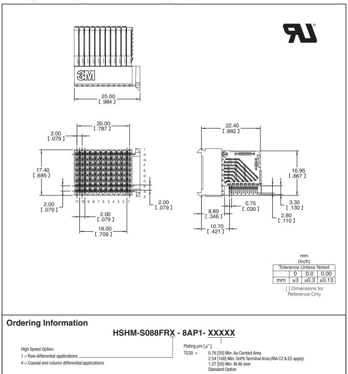
0.76 [30] Min. Au Contact Area, Lubricated TG30L =
