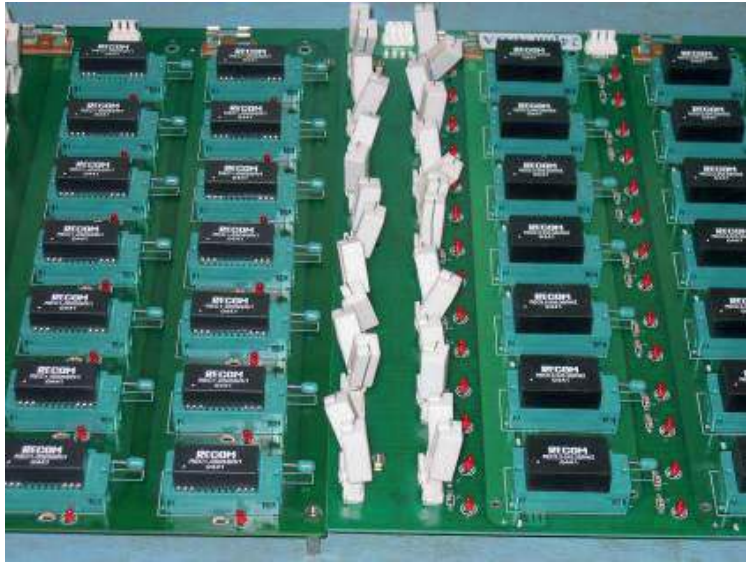
Fig. 7.2: DC/DC converters being tested in a burn-in chamber ( T_{AMB} = 40^{\circ}\text{C} )
