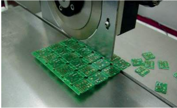
Fig. 7.4: V-Cut machine being used to singulate the PCB boards
