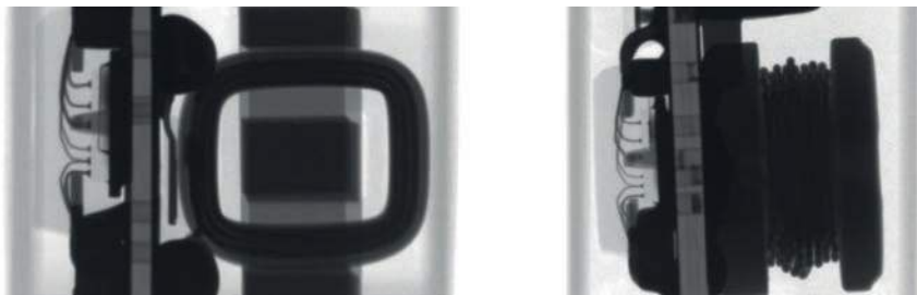
Fig 7.18: X-ray comparison between the shielded inductor used in RECOM’s R-78 switching regulator (left image) and the unshielded inductor used in a competitor’s copy product (right image).
