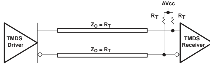
Figure 1. Termination for TMSD Output Driver
