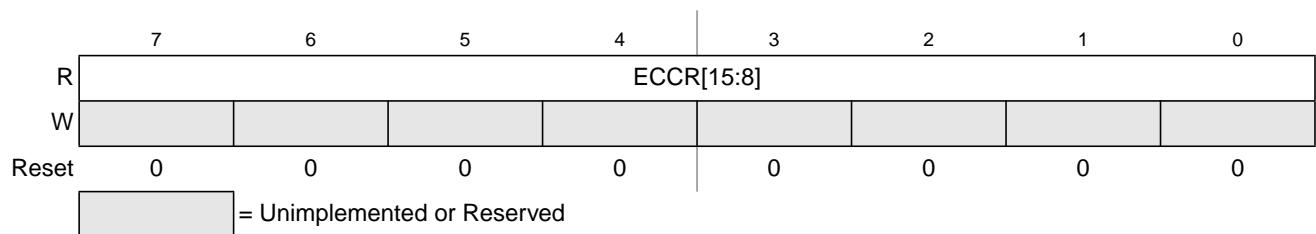
Figure 18-20. Flash ECC Error Results High Register (FECCRHI)
