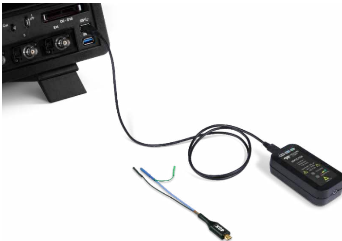
Amplifier recharging from oscilloscope USB port.
