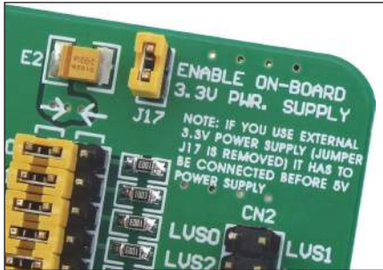
Figure 7: Jumper J17 placed on the board
