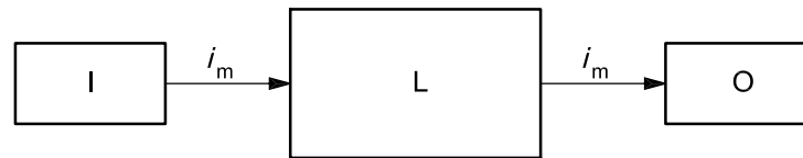
Figure 37 - Designated architecture for Category 1 (EN ISO 13849-1)
