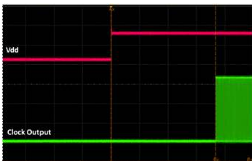
Figure 17. Startup Waveform vs. Vdd
