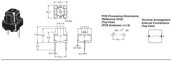
Note: Unless otherwise specified, a tolerance of ±0.4 mm applies to all dimensions. No terminal numbers are indicated on the Switches.
