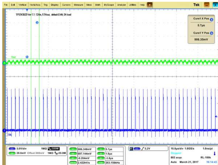
Figure 9-6. Output Ripple and SW Node of 0.9-V Output at 12-V IN , 0-A Output
