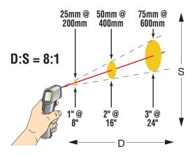
The MiniTemp thermometer is intended for close range targets, measuring a minimum target area of 1 inch in diameter out to a distance of approximately 8 inches, and has a 6 inch target measurement area at 4 feet.
