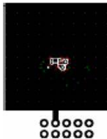
a) 200 ^\circ\text{C}/\text{W} when mounted on a 1 in 2 pad of 2 oz copper.
