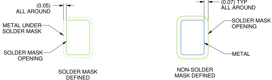
SOLDER MASK DETAIL
