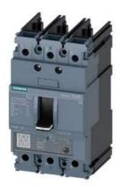
circuit breaker 3VA5 UL frame 125 breaking capacity class S 25kA @ 480V 3-pole, line protection TM230, FTAM, In=110A overload protection Ir=110A fixed short-circuit protection Ii=5...10 x In UL 489 SB (naval), 50° C without connection
