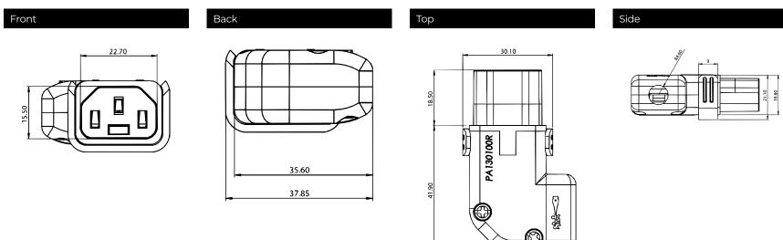
All dimensions in mm; 1 inch = 25.4 mm Tolerances according: ISO 2768-m/EN 22768-m
