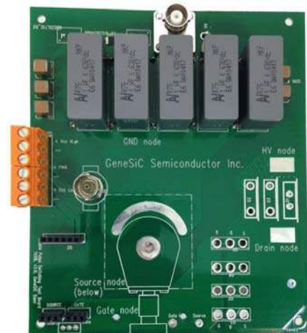
Figure 1: Double Pulse Test Board
