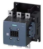
power contactor, AC-3e/AC-3 300 A, 160 kW / 400 V, without operating mechanism 3-pole, auxiliary contacts 2 NO + 2 NC main circuit: busbar control and auxiliary circuit: screw terminal
