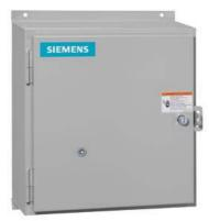
2-speed 3-phase motor starter, Size 2, One winding consequent pole, Constant or variable torque, Solid-state overload relays, Low Spd OLR range 13-52A, High Spd OLR range 13-52A, Encl. NEMA type 4X fiberglass, Water/dust tight noncorrosive
