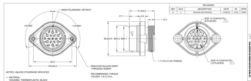
2. MODIFICATIONS: WIDE THREAD ADAPTOR (WTA); REDUCED DIA. WIRE SEAL SEALED PANEL MOUNT
