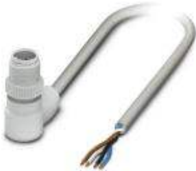
Sensor/Actuator cable, 4-position, PP-EPDM halogen-free, Gray RAL 7035, Plug angled M12, A-coded, on Free cable end, Cable length: 1.5 m, Hygienic design, with plastic knurl
