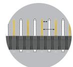
Selectively loading contacts achieves customer specific creepage and clearance requrements.
