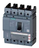
circuit breaker 3VA5 UL frame 250 breaking capacity class C 100kA @ 480V 4-pole, line protection TM210, FTFM, In=90A overload protection Ir=90A fixed short-circuit protection Ii=10 x In N conductor protection 100% without connection
